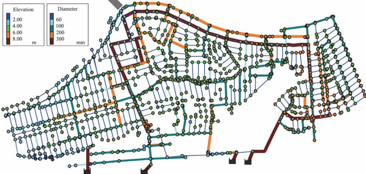
Fig. 2. Bessa network in EPANET
